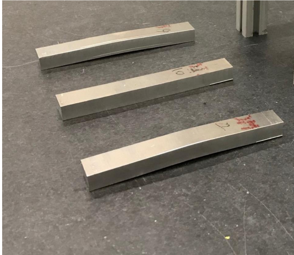
Figure 116 All three samples are displayed after applying bending and torsion forces with top, middle, and bottom samples as 14, 10, and 22 respectively
