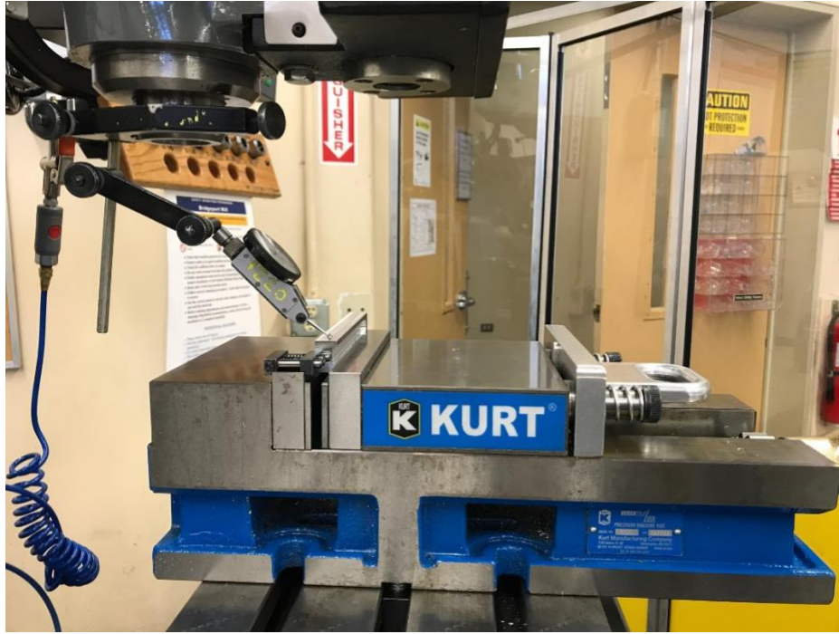
Figure 93 A dial indicator is used to measure deflection of thin walled aerospace workpieces in between milling passes at designated constant incremental locations
