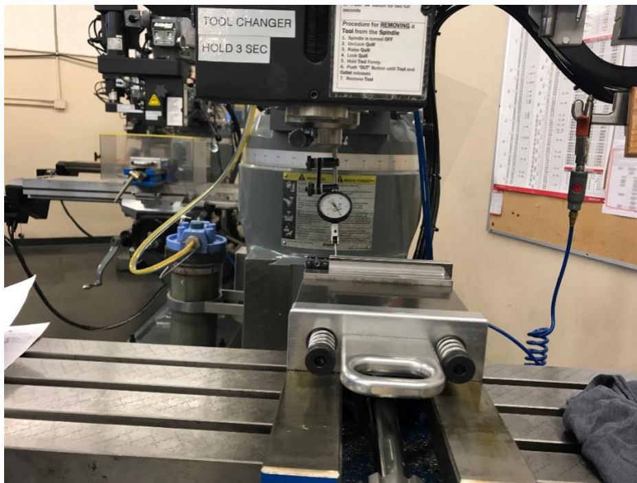
Figure 94 A front view of a dial indicator is used to measure deflection of thin walled aerospace workpieces
