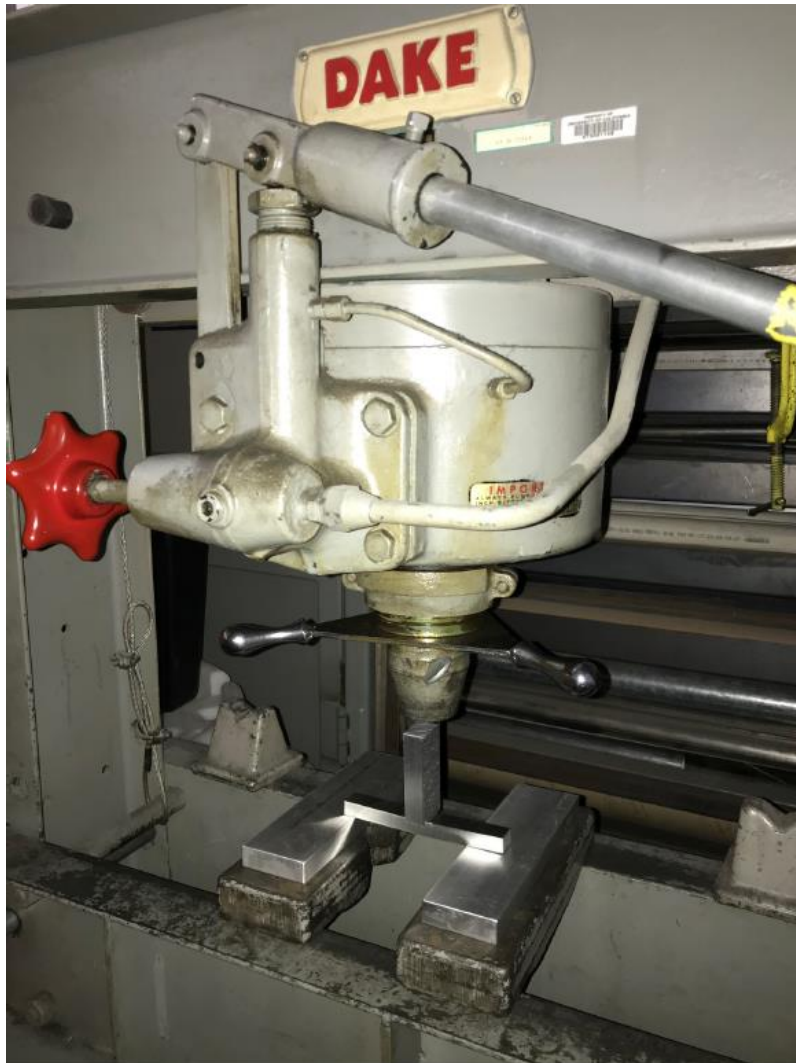
Figure 114 A Dake Hydraulic Press is displayed exerting force on a distortion sample
