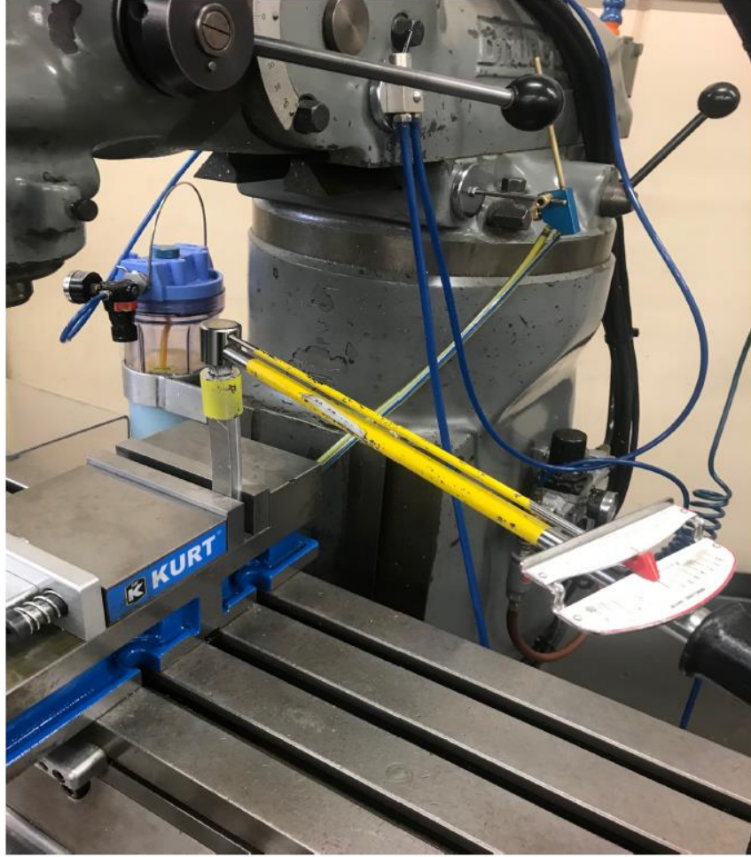
Figure 115 A craftsman torque wrench is displayed exerting torsion onto a distortion sample
