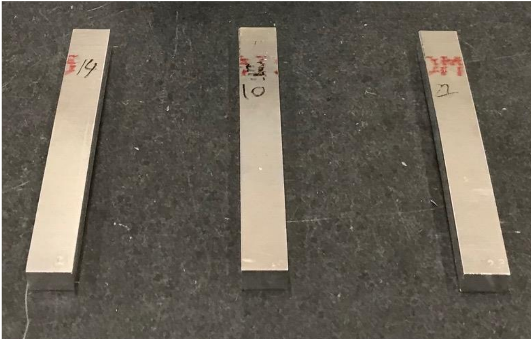
Figure 113 Al 7050 samples with induced bending, twisting, and combined bending and twisting distortions
