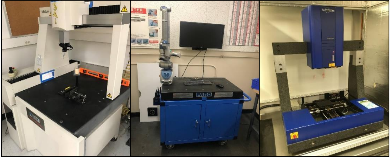
Figure 40 Three coordinate measuring machines are introduced from left to right as the Mitutoyo Bright BRT 504 CMM (left), Faro Arm Edge and Scan Arm HD CMM (middle), and the Taylor Hobson Talyscan 250 CMM (right)
